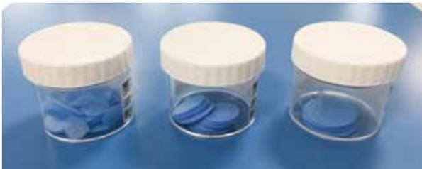
Lens paper disks are an excellent support for freezing small fragments or delicate specimens making the difficult task simple and rapid. Available in 3 sizes (diameters of 16, 22, 30 mm diameters).
